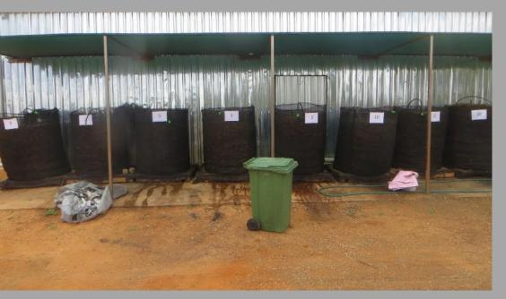
The amounts of crushed biochar added to each of the eight reactors are 0, 1, 2, 3, 5, 10, 15 and 20% of the volume, to hopefully determine the optimum. Will be ready for testing in Jan 2020
