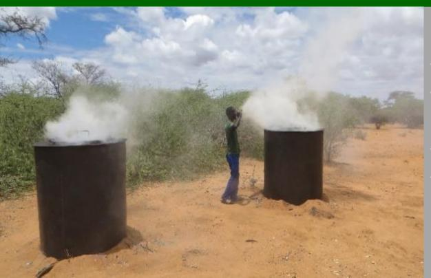
One type of charcoal tested as biochar is from the common drum kiln, comprising the "fines" that fell through the finest sieve, which gets sold at a low price
