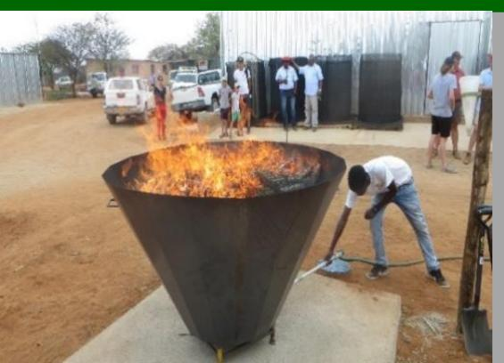
Water was used to quench biochar produced in a Kon-Tiki kiln at CCF
