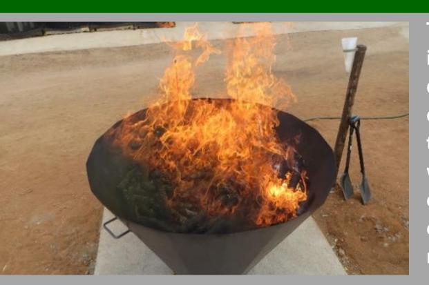
The other was produced in a Kon-Tiki kiln, designed for improved efficiency at higher temperature that burns with a clean flame, clearing tar and oils from char pores, enhancing microorganisms
