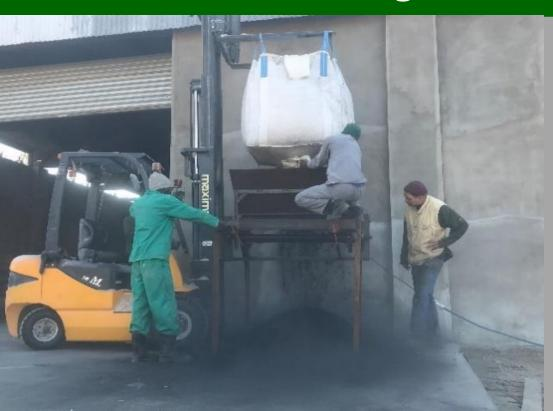
The Kon-Tiki char is crushed between rollers
